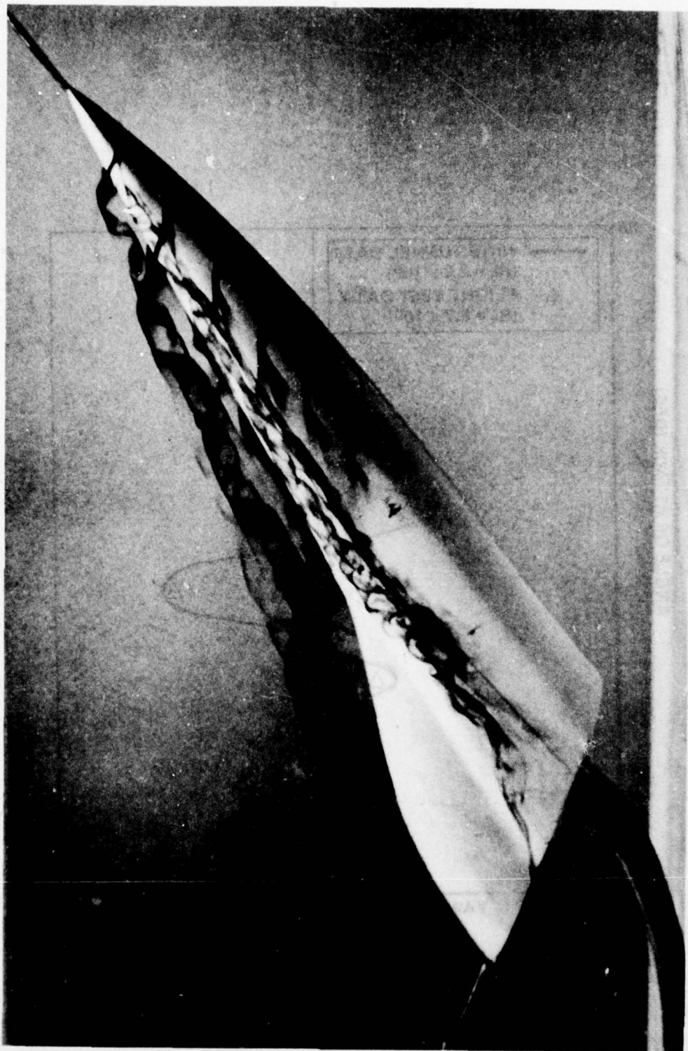
Figure 9. F-5F Forebody in Water Tunnel
