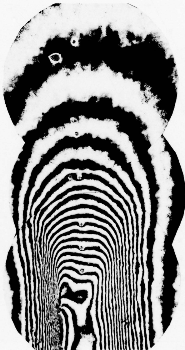
Figure 12. Interference Pattern of the Residual Deformation Field Surrounding the Crack Tip. Micrograph Was Obtained Using a Zeiss Interference Microscope
