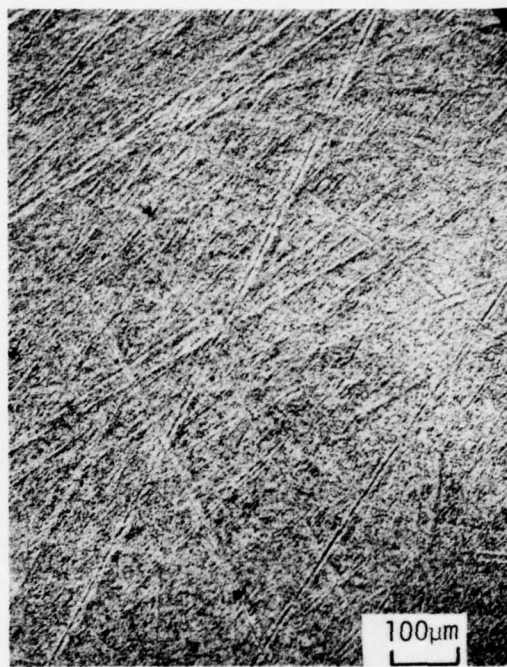
b) Dislocation Etched Impact Site for Shot No. 1010. Note Absence of Fracture Annulus.
