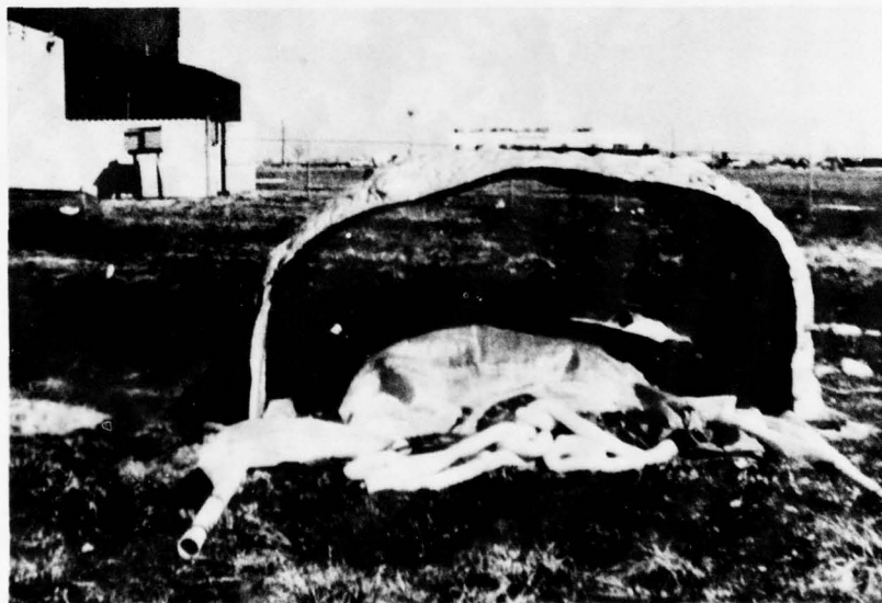
Figure 2. Foam structure produced from multiple tube membrane. Note sag and flatness of roof.
