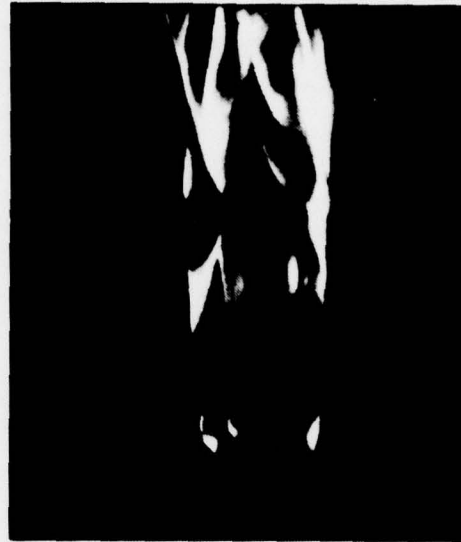
Figure 4. Single frame from high-speed cine camera, 1000 fps, 8D < x < 16D showing separate ring vortex flames and streak formation.
