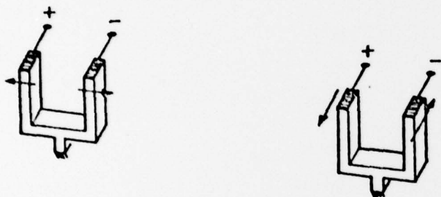
FIGURE 1. A Conventional flexural tuning fork resonator is shown in the upper left and a "face-shear" analogue in the upper right. The bottom of the figure shows a primitive horizontal shear grating resonator realized by stacking "face-shear" tuning forks.
