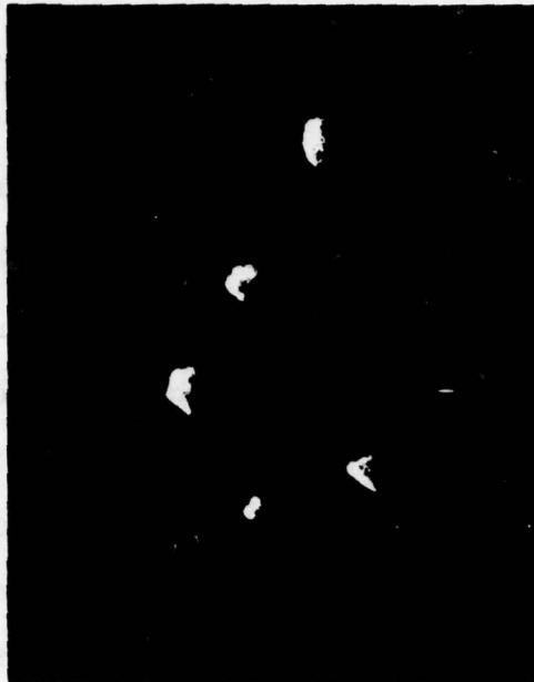
Figure 19. Secondary Electron Micrograph of Faceted Gold Islands Present in Sputter Etched Region of Target PAR 1(11)-2 After 375 °C Bake. The gold regions are several microns in diameter.
