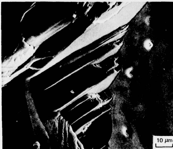
Figure 8. SEM photomicrograph of molybdenum/single crystal \text{Al}_2\text{O}_3 parted along the molybdenum wire screen plane.
