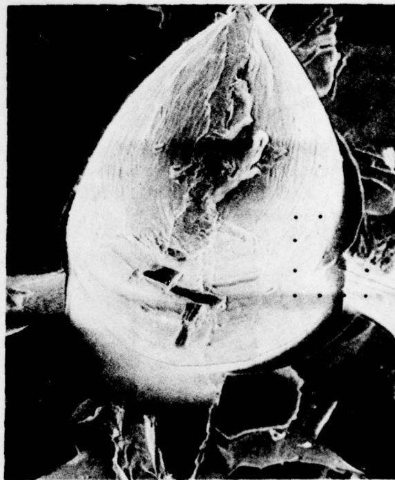
b. SEM of molybdenum wire (labeled 2) fracture; wire = 0.007'' diameter
