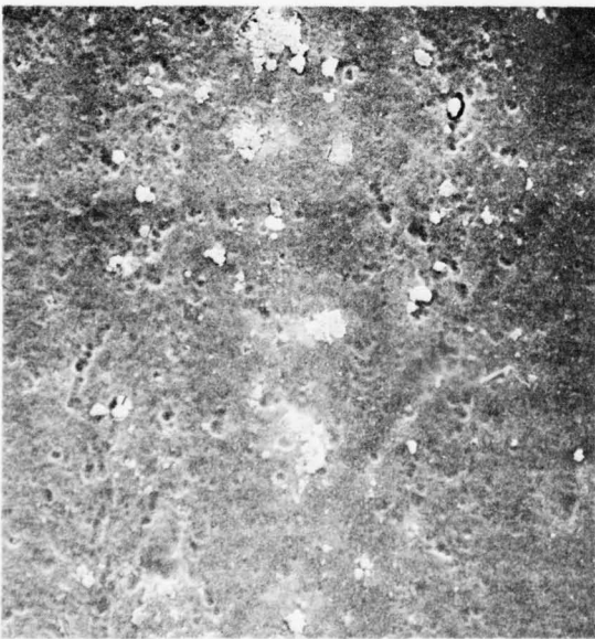
FIGURE 27. CONTAMINATION PRESENT ON A 2024-T3 ALCLAD SAMPLE DEOXIDIZED IN A 11% \text{HNO}_3 - 3.2% AMCHEM-7 BATH MODIFIED WITH ALODINE-45, 2 ml/l (ETCH RATE 0.200 mils/side/hour)
