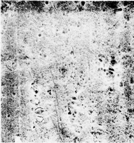
FIGURE 22. INADEQUATE SURFACE ETCHING OF A 7075-T6 BARE SAMPLE DEOXIDIZED IN A 9% \text{HNO}_3 - 3.2% AMCHEM-7 BATH
