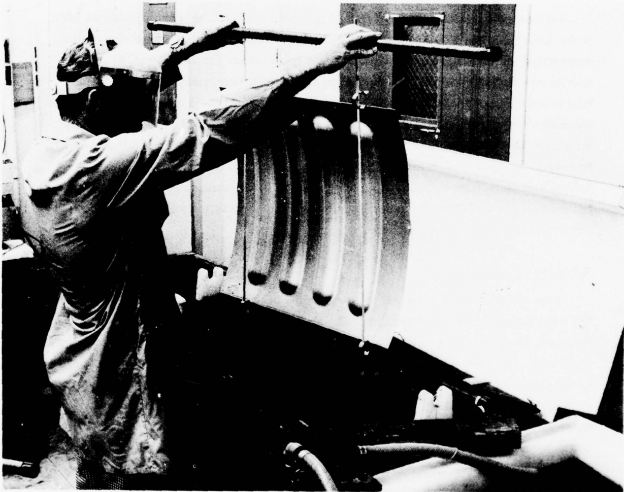
FIGURE 106. PANEL MOUNTED IN SURFACE PREPARATION FIXTURE
