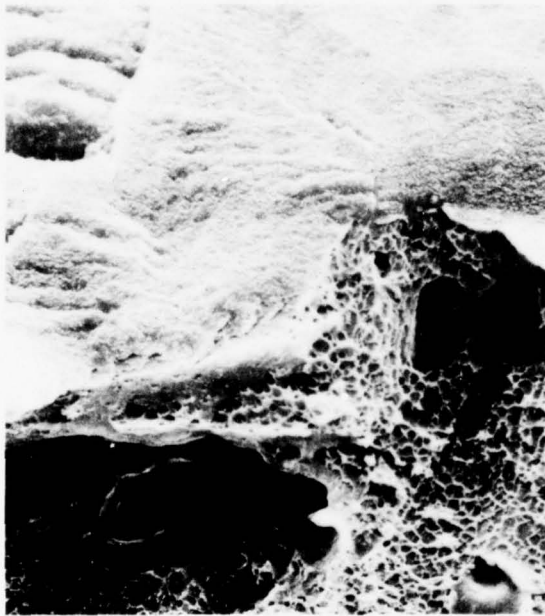
FIGURE D4. GENERAL SURFACE CHARACTERISTICS OF THE AREA USED FOR OXIDE THICKNESS DETERMINATION OF BARE 7075-T6 ANODIZED IN PHOSPHORIC ACID/SODIUM DICHROMATE
