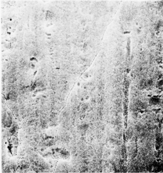
FIGURE 24. DEGREE OF ETCHING IN A 7075-T6 BARE SAMPLE DEOXIDIZED IN A 11% \text{HNO}_3 - 3.2% AMCHEM-7 BATH
