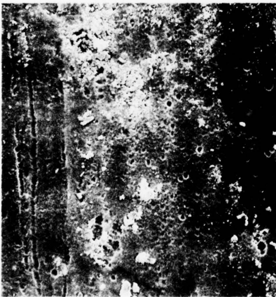
FIGURE 23. CONTAMINATION PRESENT ON 2024-T3 ALCLAD DEOXIDIZED IN A 9% \text{HNO}_3 - 3.2% AMCHEM-7 BATH
