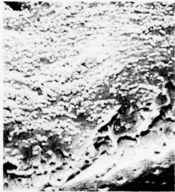
FIGURE D4. GENERAL SURFACE CHARACTERISTICS OF THE AREA USED FOR OXIDE THICKNESS DETERMINATION OF BARE 7075-T6 ANODIZED IN PHOSPHORIC ACID/SODIUM DICHROMATE
