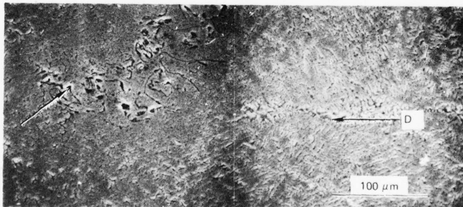
c. HIGHER MAGNIFICATION OF PART OF AREA (b). ARROW TO LEFT INDICATES POSSIBLE TRAPPED ADHESIVE.
