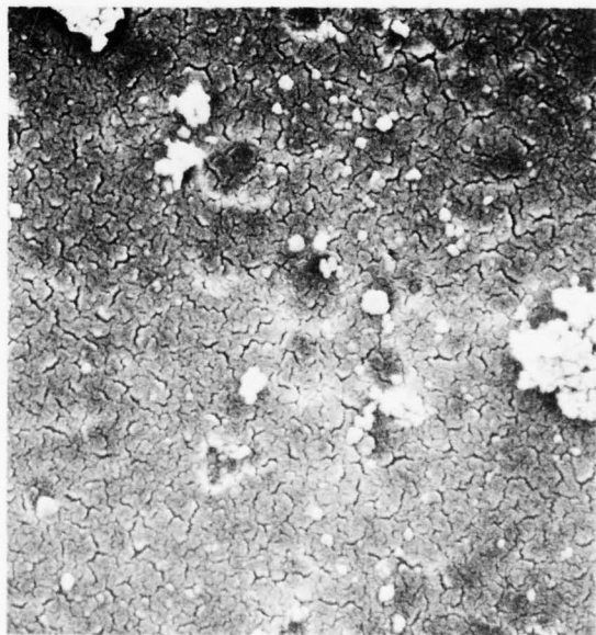
FIGURE 27. CONTAMINATION PRESENT ON A 2024-T3 ALCLAD SAMPLE DEOXIDIZED IN A 11% \text{HNO}_3 - 3.2% AMCHEM-7 BATH MODIFIED WITH ALODINE-45, 2 ml/l (ETCH RATE 0.200 mils/side/hour)
