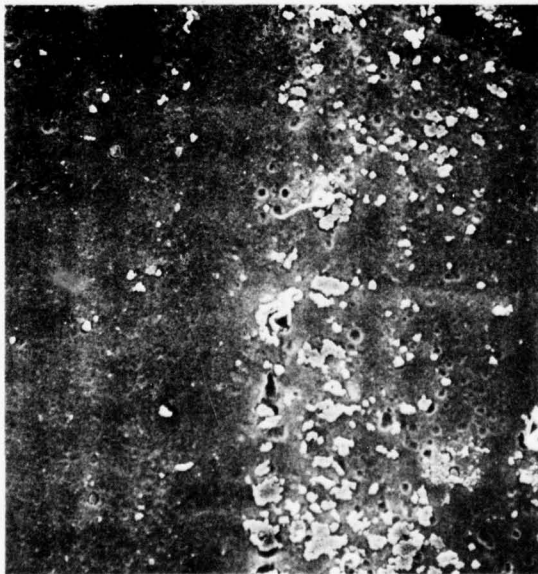
FIGURE 25. CONTAMINATION PRESENT ON 2024-T3 ALCLAD DEOXIDIZED IN A 11% \text{HNO}_3 - 3.2% AMCHEM-7 BATH
