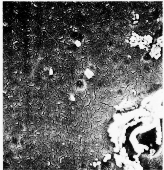
FIGURE 25. CONTAMINATION PRESENT ON 2024-T3 ALCLAD DEOXIDIZED IN A 11% \text{HNO}_3 - 3.2% AMCHEM-7 BATH
