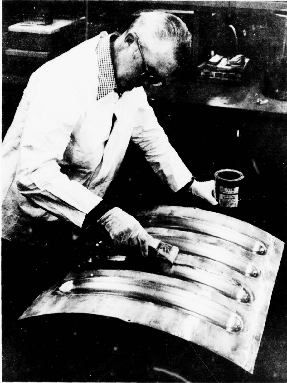
FIGURE 133. APPLYING A-1444B PASTE ADHESIVE TO BEADED PAN DETAIL
