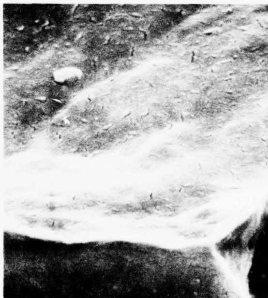
FIGURE D5. GENERAL CHARACTER OF STANDARD SURFACE OF 2024-T3 ALCLAD "DEOXIDIZED ONLY"
