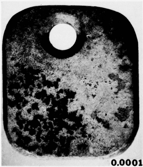
Figure 5. Effect of \text{SO}_2 pressure on 704C sulfate-induced hot corrosion of aluminized (PWA 28) Mar-M509, as shown by surface condition after 20 hours and weight change data for 100-hour cyclic exposure.
