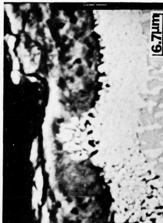
Figure 36. Microstructures of PWA 68 CoCrAlY coating tested at 704C with simultaneous presence of gaseous \text{SO}_3 (0.0007 atm) and NaCl vapor (30 ppm). Note characteristic morphology of both \text{SO}_3 - and NaCl-induced hot corrosion in randomly selected areas of the attack front.
