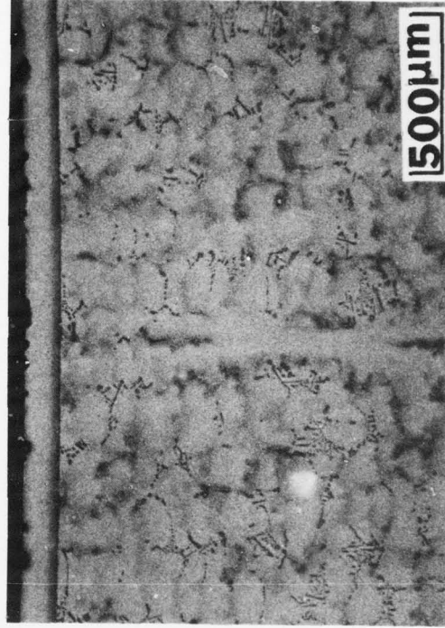
Exposed 20 hours; 704C, P SO 3 = 0.0007 atm
