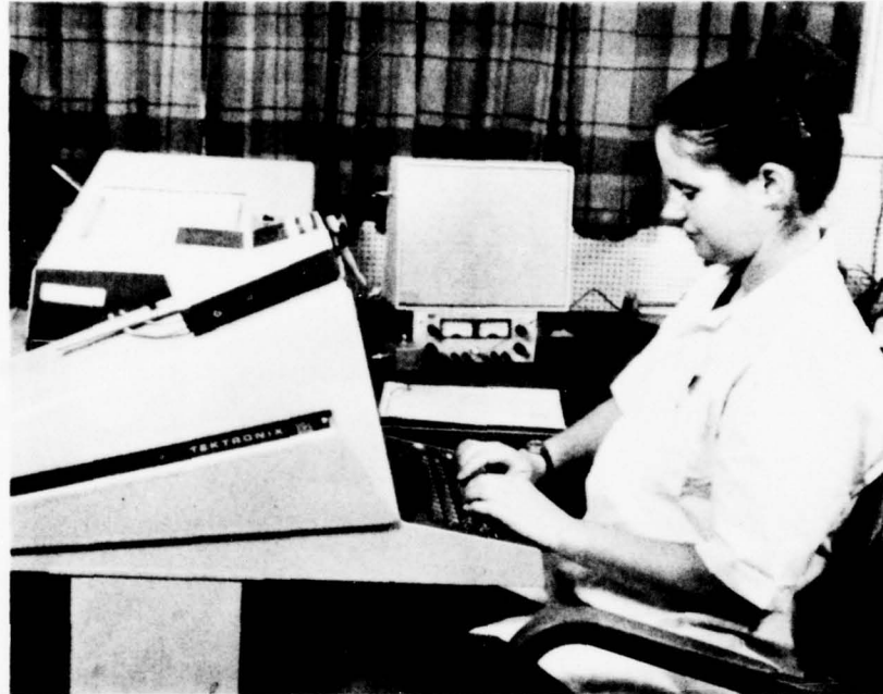
FIGURE 13. Terminal operator initializes computer program, monitors computer operations, notifies test personnel of error messages, and insures completeness of "quick-look" data at the end of each data trial. Hard copy of data is generated at this position also.
