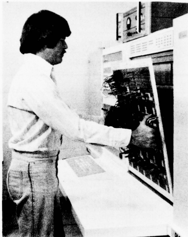
FIGURE 15. Computer programmer inserts program board into PACER 600 Analog Computer. The Analog Computer, under control of the SEL 8500 Digital Computer, controls moving target system (MTS), data acquisition, Multi-Axis Helicopter Vibration System (MAHVS), and monitors all control functions and indicators.
