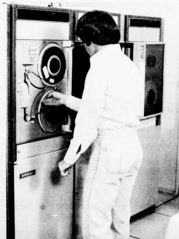
FIGURE 16. Computer programmer mounts tape to collect digitized aiming/tracking data generated during experiment.
