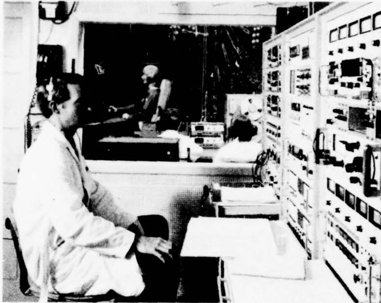
FIGURE 14. The Multi-Axis Helicopter Vibration Simulator (MAHVS) operator monitors system performance. In the event of a system malfunction, the operator must disarm hydraulic systems, correct deficiency, and reinitialize simulator. Controller, timekeeper, and subject stations shown in background.
