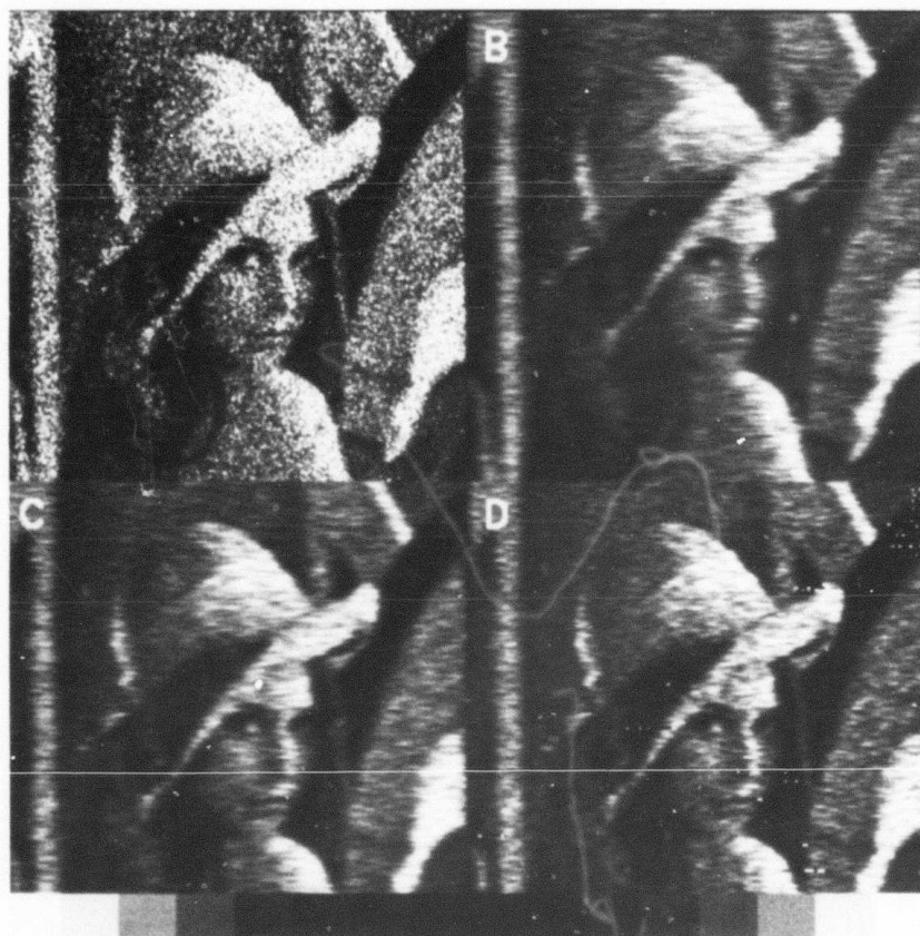
Figure 5.7 Restored images with a global adaptive MAP filter for \frac{(\text{SNR})_{\text{rms}}}{\sqrt{10}}
