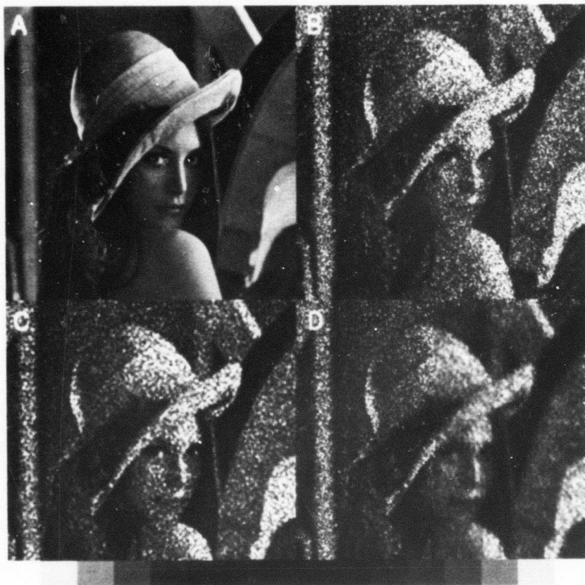
Figure 7.3d Images restored by the LMMSE filter and the MAP filter with two-dimensional linear blurring degradation at \overline{(\text{SNR})}_{\text{rms}} = \sqrt{20}
