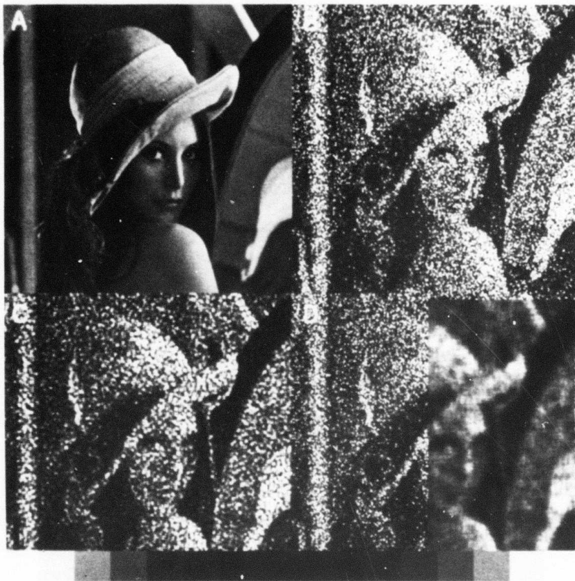
Figure 7.3b Images restored by the LMMSE filter and the MAP filter with two-dimensional linear blurring degradation at (\text{SNR})_{\text{rms}} = \sqrt{5}
