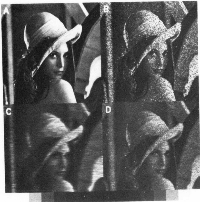
Figure 4.1c Restored image with a MAP filter with R_f = \sigma^2 I and \frac{(SNR)_{rms}}{rms} = \sqrt{20}
