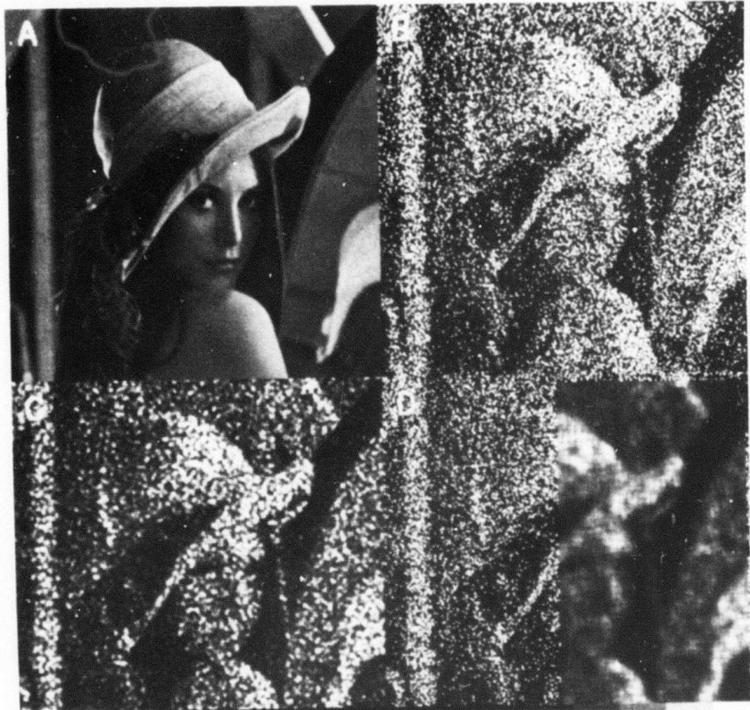
Figure 7.3a Images restored by the LMMSE filter and the MAP filter with two-dimensional linear blurring degradation at (\text{SNR})_{\text{rms}} = \sqrt{2.5}
