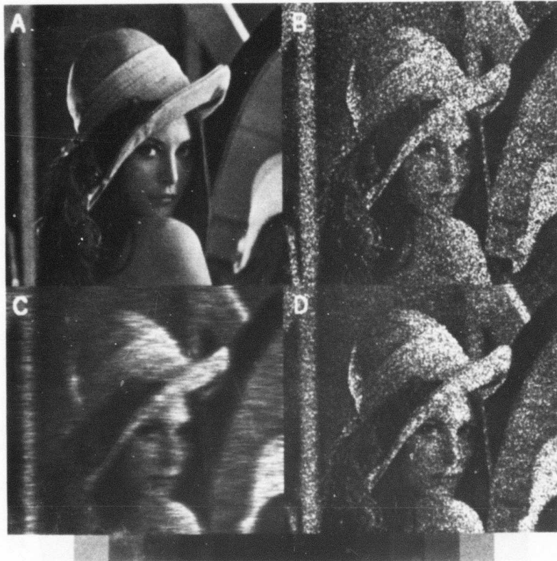
Figure 4.1b Restored image with a MAP filter with R_f = \sigma^2 I and \frac{(\text{SNR})_{\text{rms}}}{\text{rms}} = \sqrt{10}
