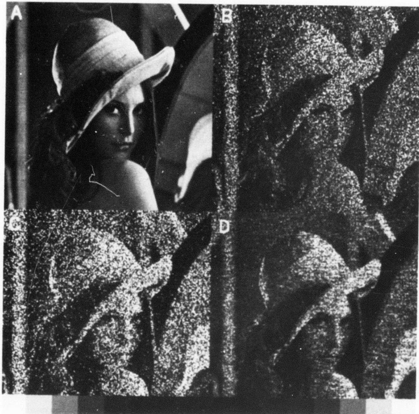
Figure 7.2b Images restored by the LMMSE filter and the MAP filter at \frac{(\text{SNR})_{\text{rms}}}{\text{rms}} = \sqrt{5}
