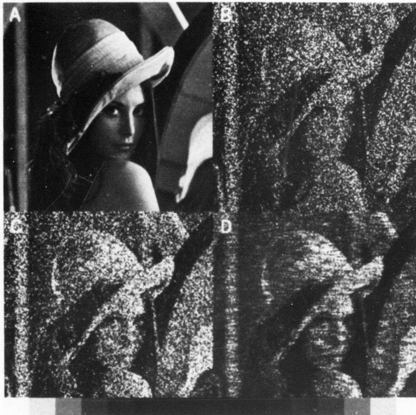
Figure 7.2a Images restored by the LMMSE filter and the MAP filter at \frac{(\text{SNR})}{\text{rms}} = \sqrt{2.5} (A) Original object image (B) Poisson noisy image (C) Image restored by the LMMSE filter (D) Image restored by the MAP filter
