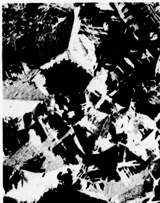
Figure 22.—Microstructures of Plate P11 in the (a) As-received (BA) Condition, and (b) and (c) BA Condition After Phase II Heat Treatment.
