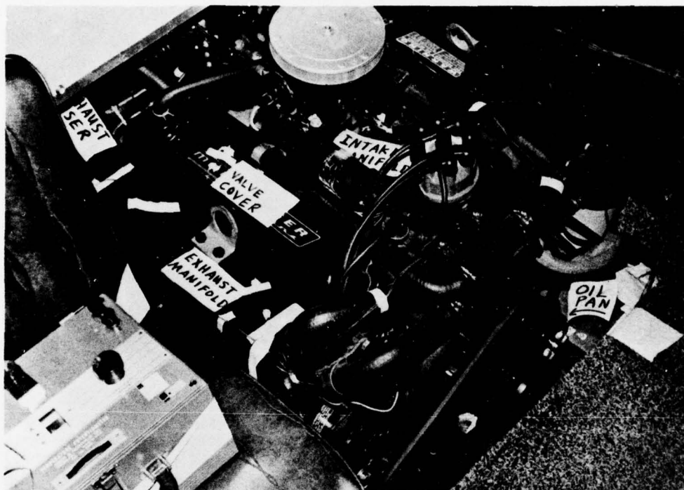
FIGURE IV-13. ENGINE COMPARTMENTS - I/O
