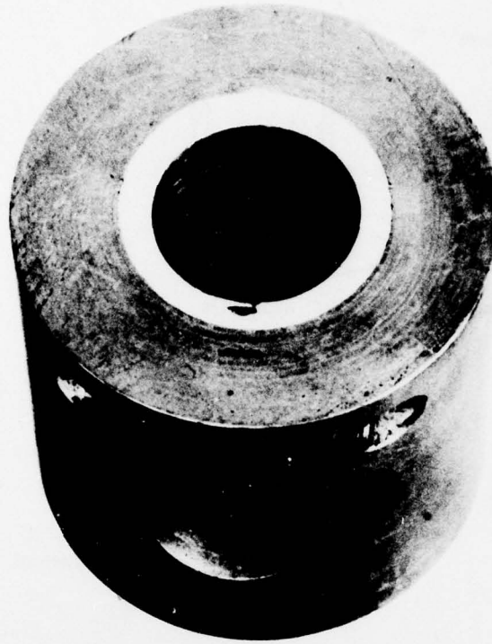
Figure A9. Photoelastic rock bolt load cell.
