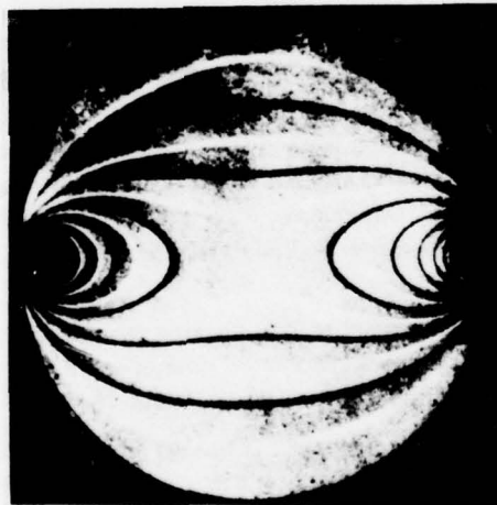
Figure 7. Sharpened isochromatic patterns for circular disk in diametral compression. (After Post 26 .)
