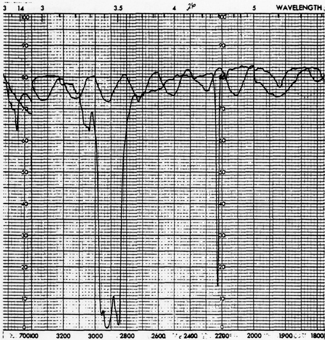
Fig. 26 Infrared (3-5 \mu m) transmission of EM ZLI-1083 phenylcyclohexane mixture (25 \mu m cell with NaCl windows).
