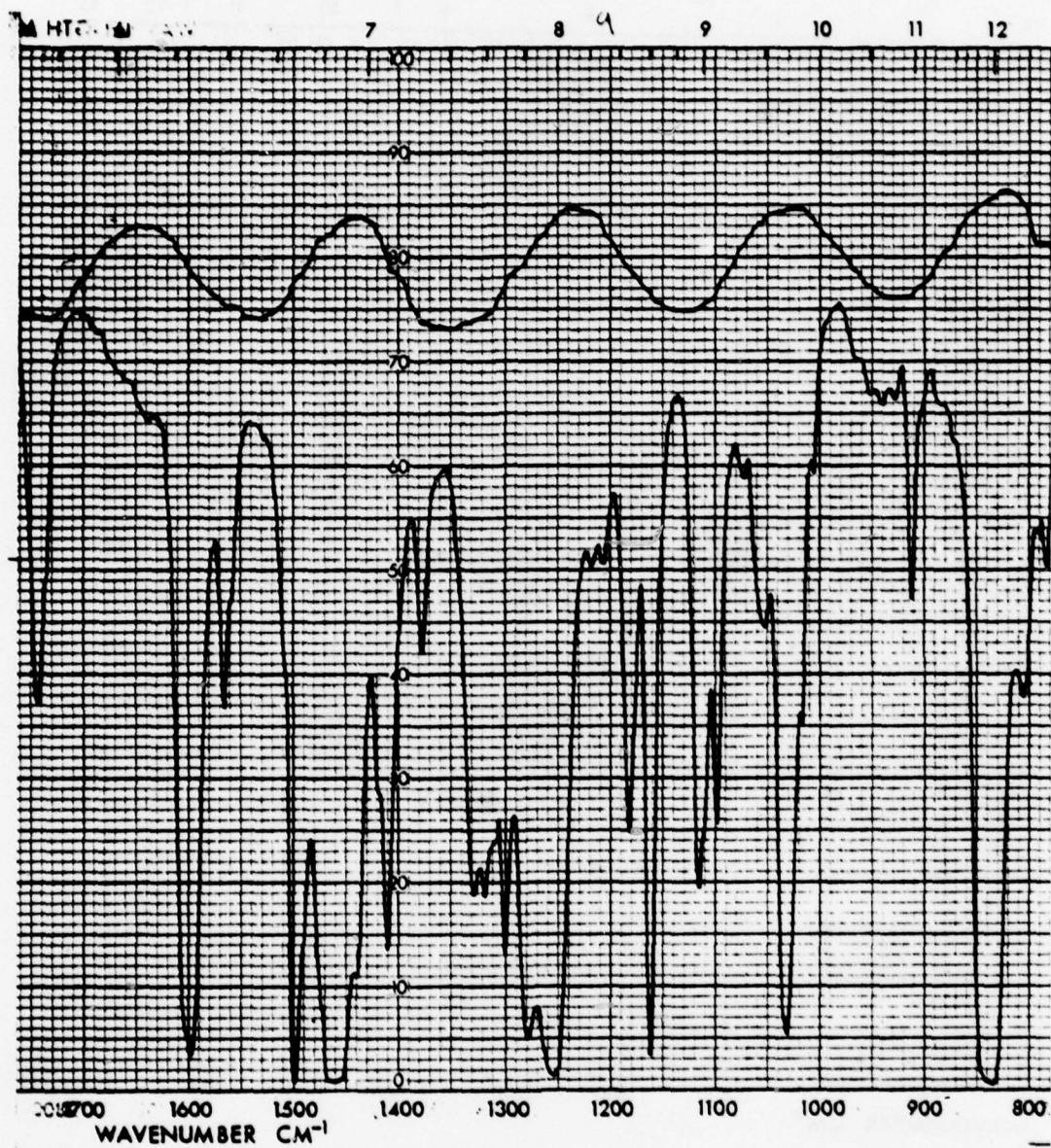
Fig. 9 Infrared (6-12 \mu m) transmission of EM Licristal azoxy and biphenyl ester mixture nematic phase 997 (25 \mu m cell with NaCl windows).
