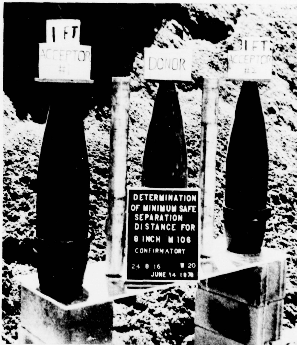
Fig 4 Shielded confirmatory test set-up
