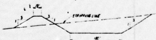
TYPICAL SECTION OF EMERGENCY SPILLWAY AND DIKE LOOKING DOWNSTREAM (SEE SHEET 18)
