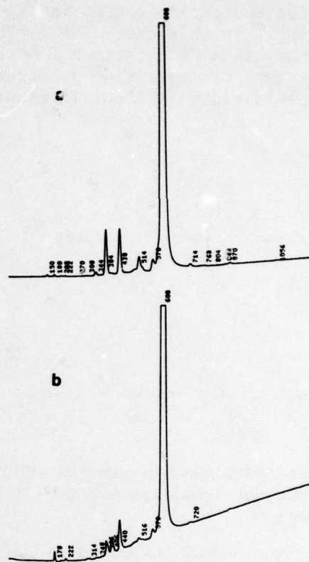
Figure 4. HPLC analysis of DDS with UV detection at (a) 280 nm and (b) 254 nm.
