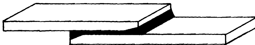
variable adhesive thickness
