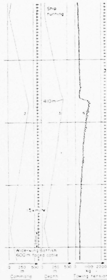
FIG. 9. Chart recording of command signal, depth, and towing tension for a wide-wing Batfish with 600 m of faired cable.
