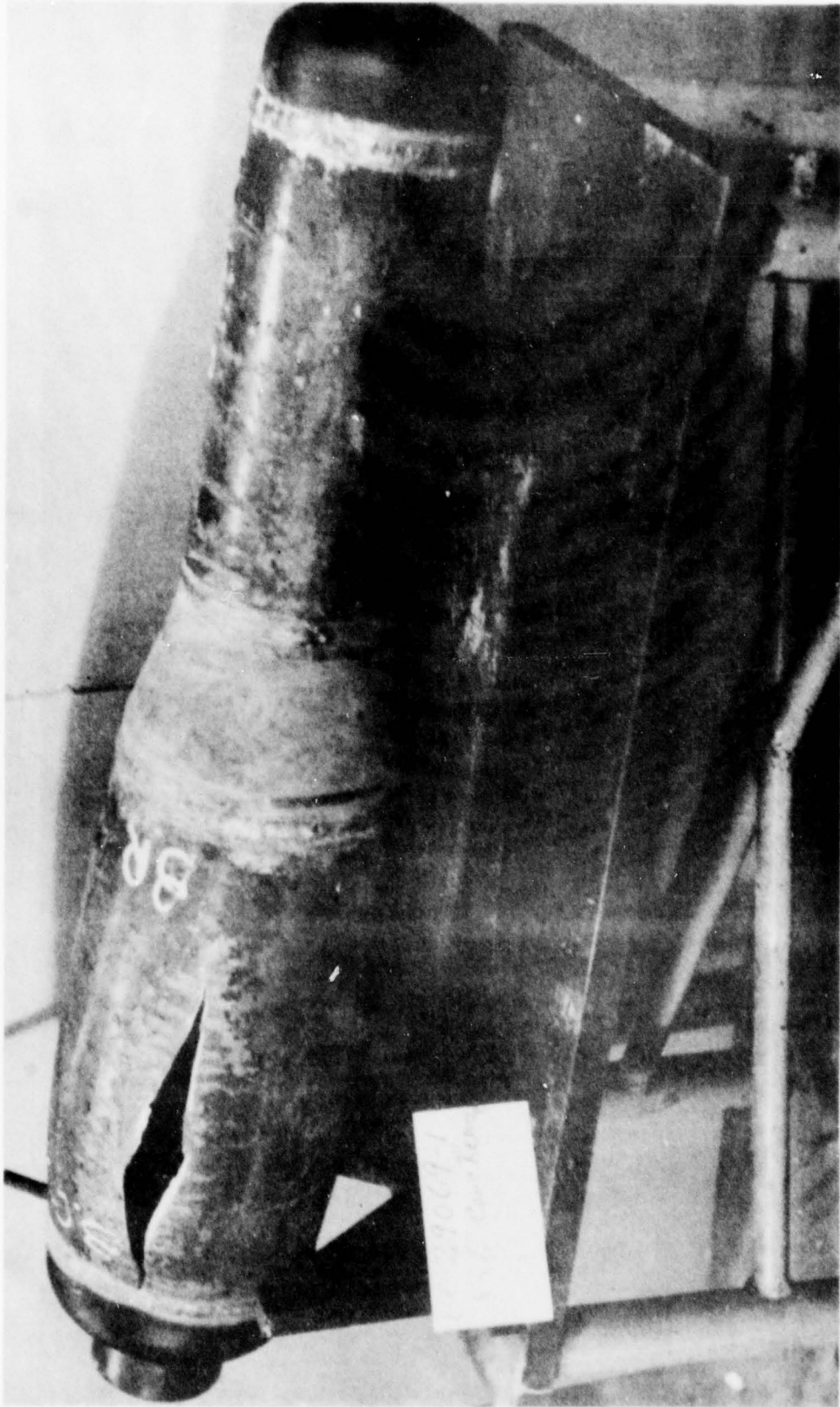
PHOTO OF 8 x 6 REDUCER TEST VESSEL AFTER FAILURE
