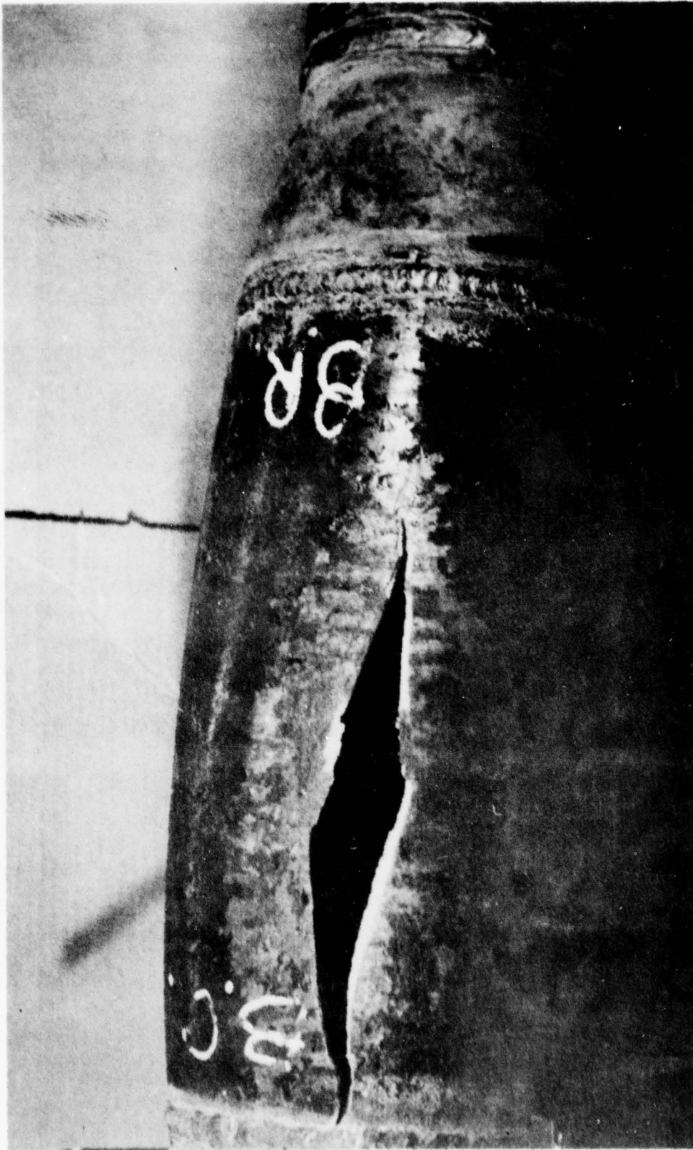
FIGURE 9 CLOSE-UP PHOTO OF FAILURE (CARBON STEEL)
