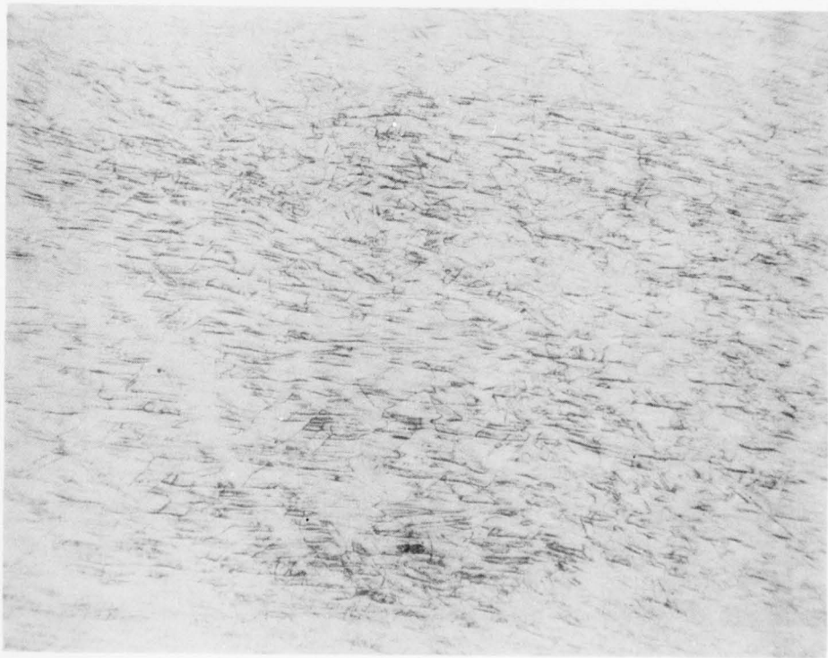
FIGURE 14 MACRO/MICRO PHOTOGRAPHS OF MIDDLE CROSS SECTION OF COPPER-NICKEL REDUCER (2X, 100X)
