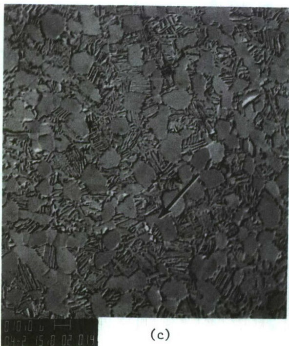
Figure 39. Microstructures of Hand Forged Billet No. 13, (a) and (b), and Die Forging No. 14, (c) and (d). Clusters of yttria particles are identified by arrows in the backscattered electron micrographs on the left and shown enlarged in the SEM's on the right.
