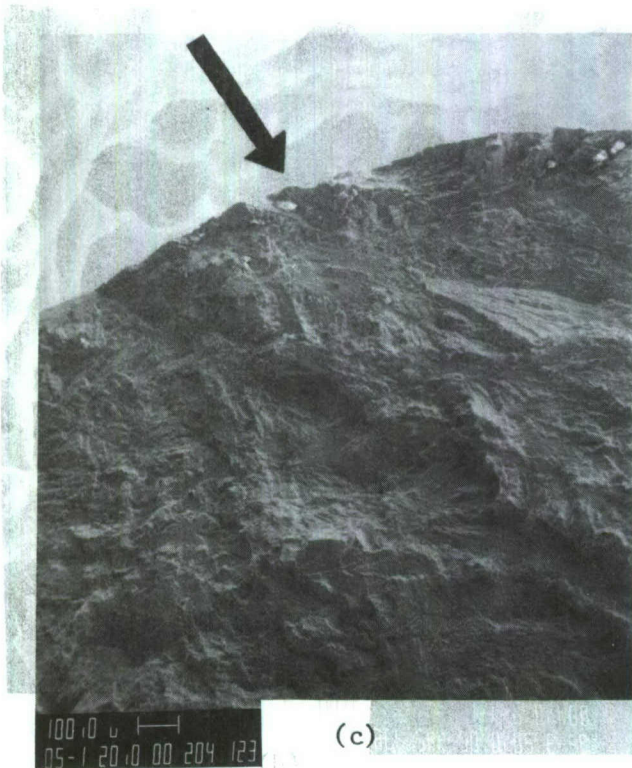
Figure 41. Scanning Electron Micrographs of the Fracture Initiation Regions of; (a) and (b) Fatigue Specimen 14-ST-16, and (c) and (d) Fatigue Specimen 12-L-4. No yttria particles were found at the multiple initiation sites; however, note the transgranular cleavage regions at each edge initiation site. The light particles are contaminants of external origin
