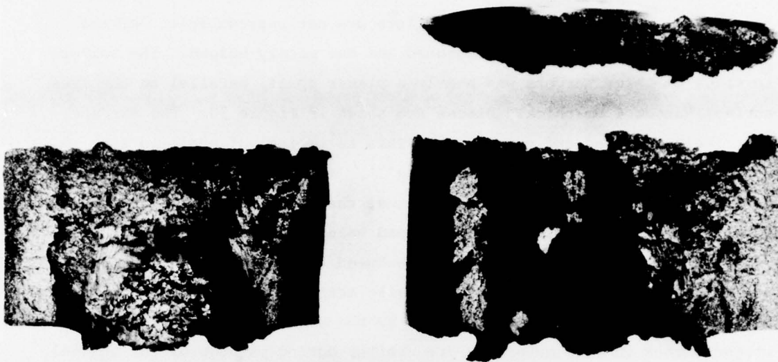
Figure 30. Post-impact Condition of a 4 cm Thick Cylinder
