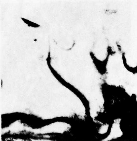
Figure 15(b). Transmission electron micrograph of \text{LaB}_6 crystal used in Figure 15(a). Magnification 48,000.
