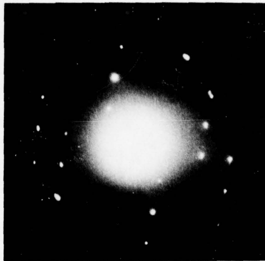
Figure 20(a). Electron diffraction pattern of the \text{LaB}_6 crystal of Figures 18 and 19.
