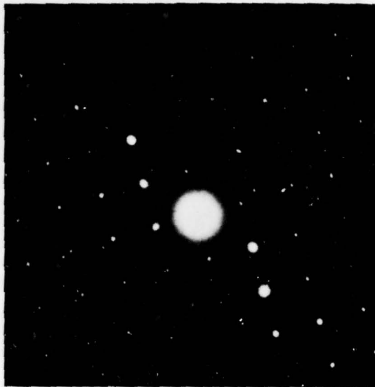
Figure 15(a). Electron diffraction pattern of \text{LaB}_6 crystal prepared by molten aluminum flux technique.
