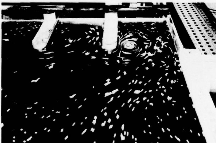
Photo 1. Surface currents during filling operation, type 1 (original) intake, time exposure 5 sec; upper pool el 750.0, lower pool el 725.0, 2.07-min valve time (sheet 1 of 2)
