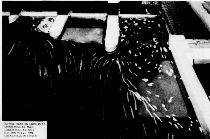
Photo 10. Type 5 (recommended) design, steady-flow peak discharge conditions through intake, time exposure 5 sec, culvert valve fully open; river discharge 14,000 cfs, discharge exceeded 11 percent of time; dam gates 1, 2, and 3 open 3.0 ft, auxiliary lock gate closed
