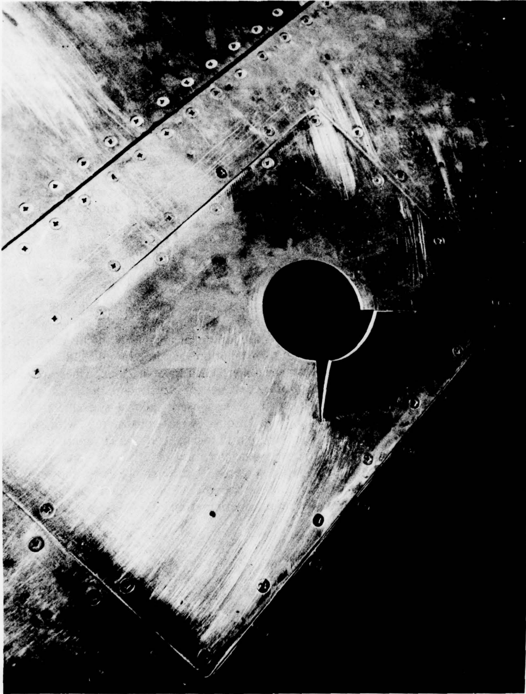
Figure 16. Leading Edge Damage.
