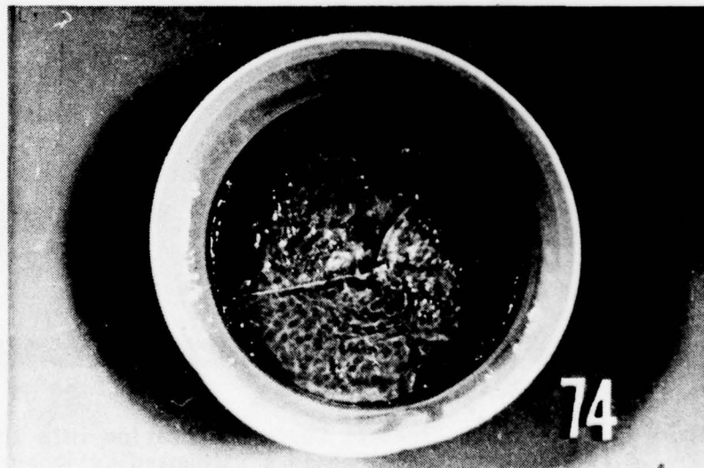
Figure 4. Thermal Crack in Neat Resin
