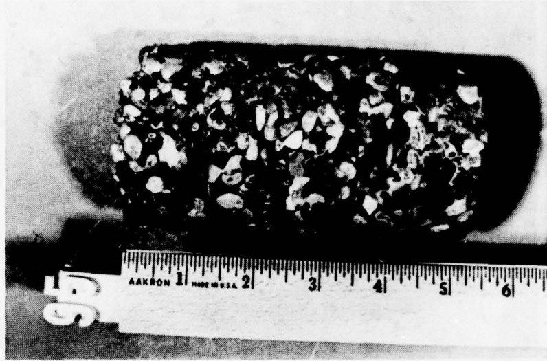
Figure 6. Varying Degrees of Resin Penetration into the Aggregate Contained in a Cardboard Cylinder (Concluded)
