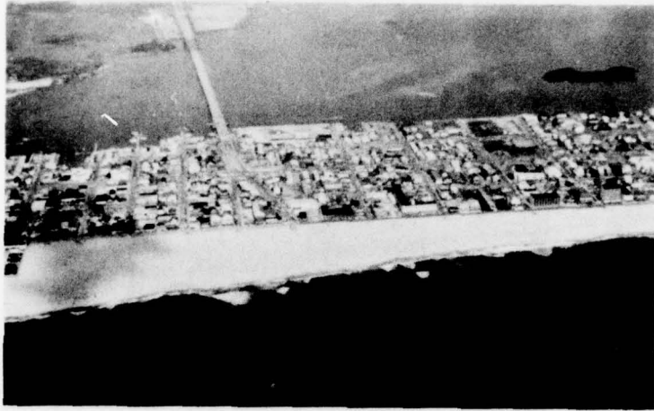
A Ocean City, Maryland, in the vicinity of the northern bridge. Note accretion toward the south (left) due to the inlet jetty.
