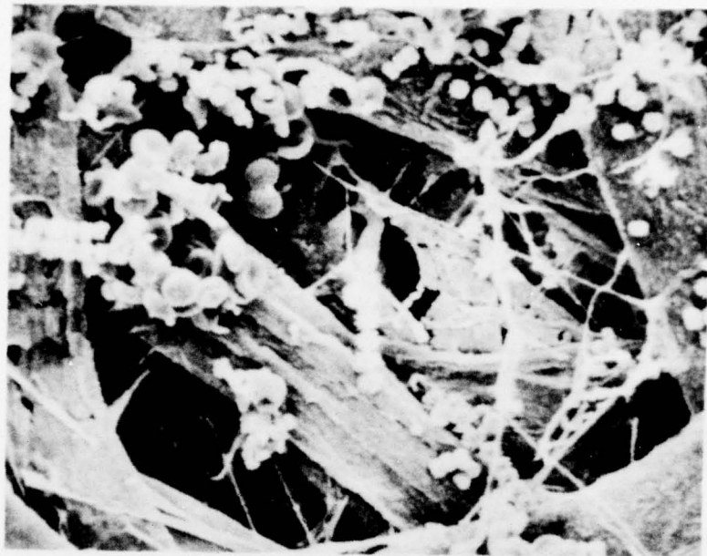
Figure 5. SEM of Fungal Growth on Underside of Outer Layer of IRT Sack No. 1
