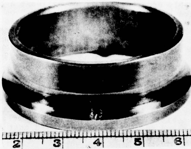
Inner Ring Bearing No. 508 47 X 10 6 Revs. (b)
