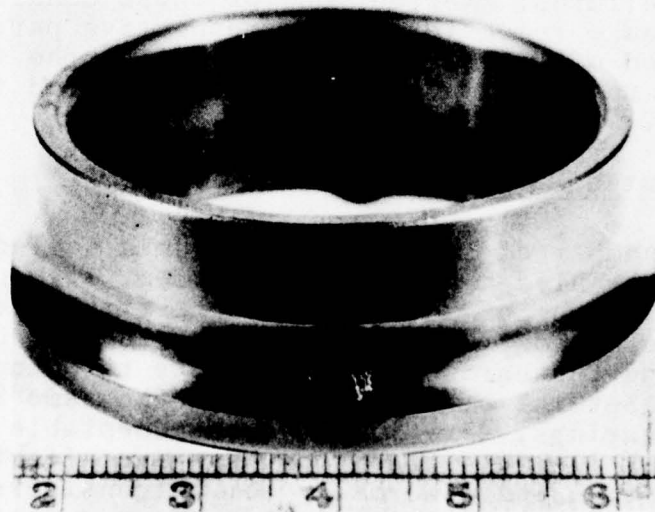
Figure 23. Typical Examples of Bearing Element Failures From 7209 VAP Angular Contact Ball Bearings
