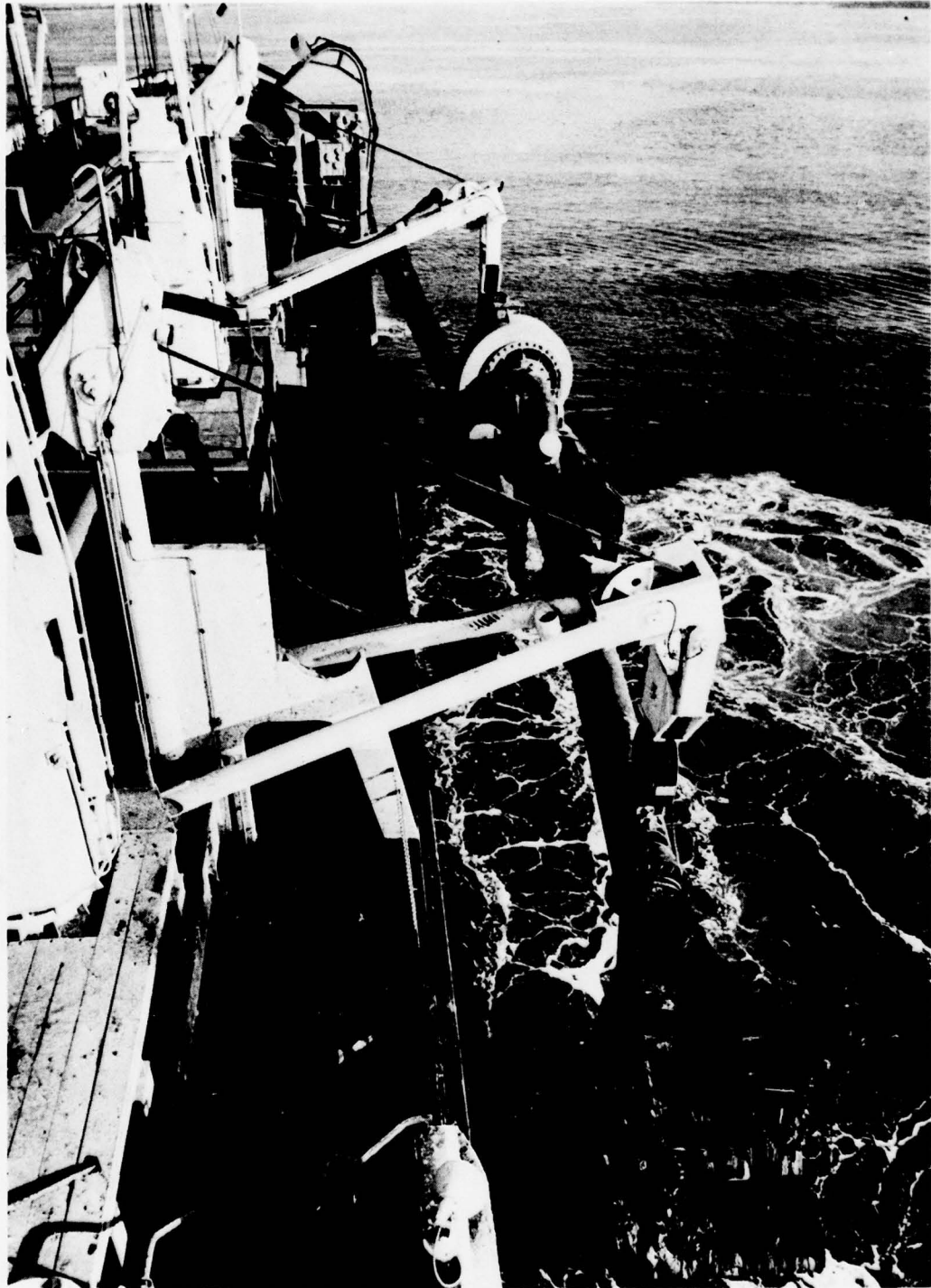
Figure 4. Pump mounted on ladder
