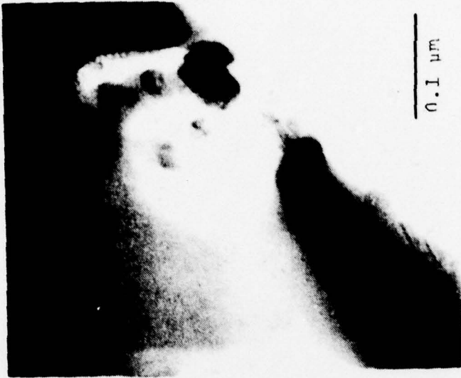
Core-sheath interface region of boron filament annealed in air at 1200°C for 3 minutes.
