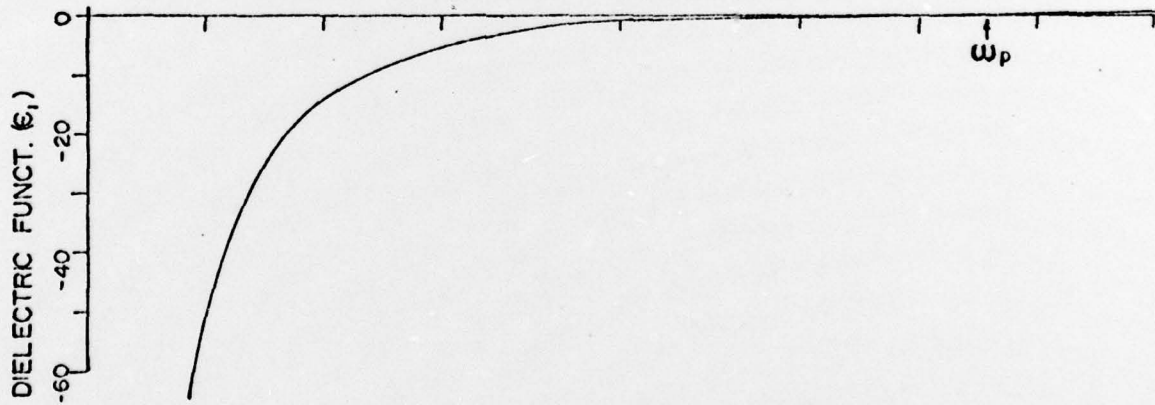
Figure 19: Extinction of aluminum calculated in the Rayleigh ellipsoid approximation for randomly oriented identical ellipsoids with shape parameters L_2 = .01, .3, .69 and for a continuous distribution of ellipsoidal shapes (CDE). The real part of the complex dielectric function, which determines the positions of the peaks, is shown below.
