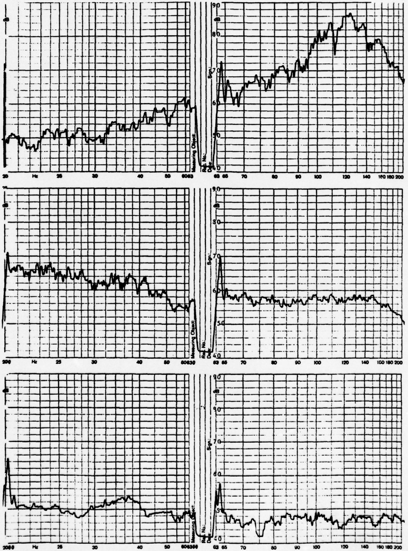
FIGURE 19. Frequency Spectrum of Rotating Diffuser From Microphone Position 1.
