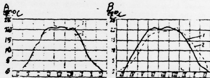
Figure 19. Long term water temperature variation curves: a - above the reservoir; b - below the reservoir; 1 - before flow regulation; 2 - after flow regulation.
