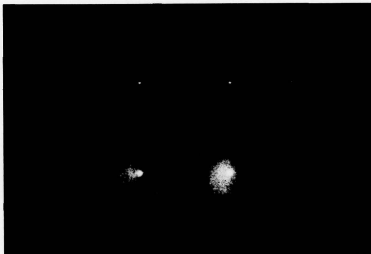
Figure 3-7. 2 x 2 ground-glass holoplex output, \beta = -1.5 , #80 grit diffuser, plane-wave illumination.
