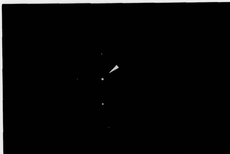
Figure 4-10. Single-point playback of element 4 (indicated by arrow) in Fig. 4-8. The other 8 terms are the crosstalk terms associated with that signal term.
