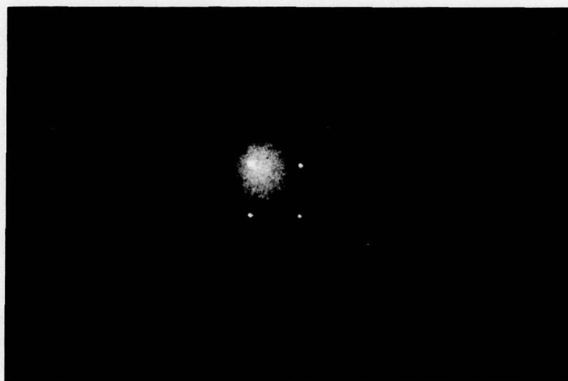
Figure 3-3. 2 x 2 ground-glass holoplex output \beta = -1/3 , #80 grit diffuser, chirped illumination.
