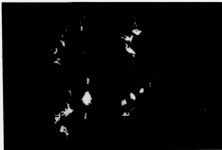
Figure 4-11. 2 x 2 shower-glass holoplex, \beta = -1.5 , shower-glass diffuser, chirped illumination, simultaneous playback.
