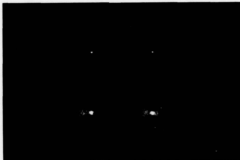
Figure 3-1. 2 x 2 Ground-glass holoplex output, \beta = -1.5 , #80 grit diffuser, chirped illumination.
