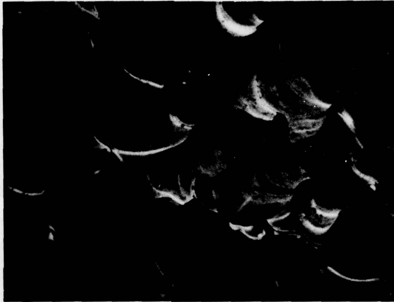
Figure 21. Microphotograph of LPE 17A Showing Poor Surface Morphology Resulting from Thermal Erosion of the Substrate Prior to Growth
