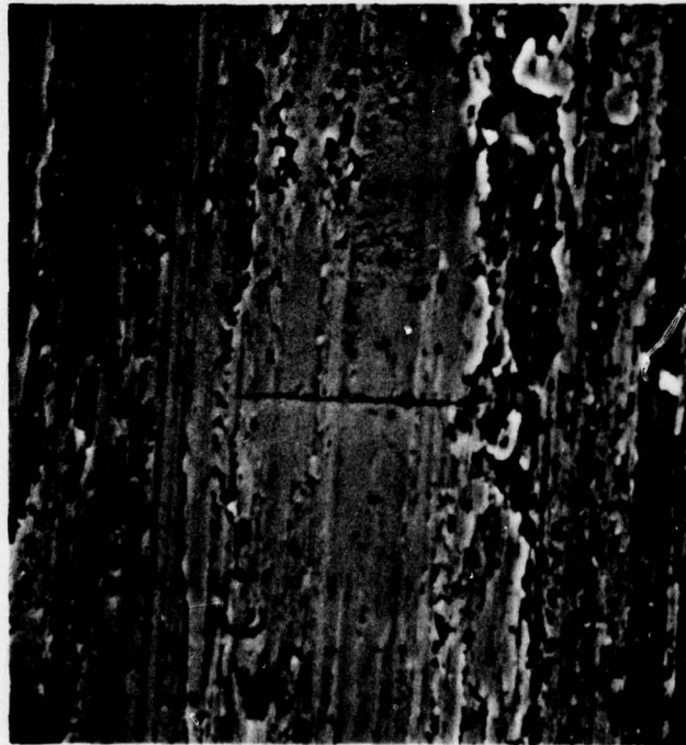
FIGURE 15. SEM MICROGRAPH OF SURFACE MICROCRACK USED IN SCOD MEASUREMENTS ON SAMPLE 8. Labeled Crack 4 (1000X).
