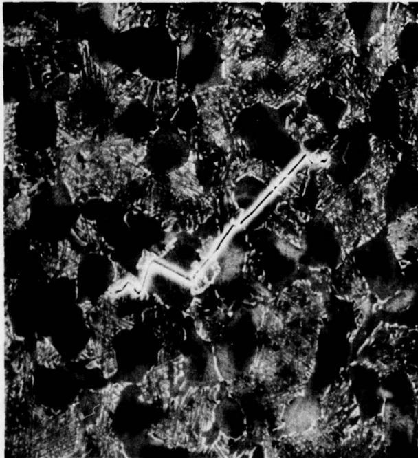
FIGURE 11. SEM MICROGRAPH OF 90 \mu\text{m} LONG SURFACE MICROCRACK USED IN SCOD MEASUREMENTS ON SAMPLE 7 (1000X)
