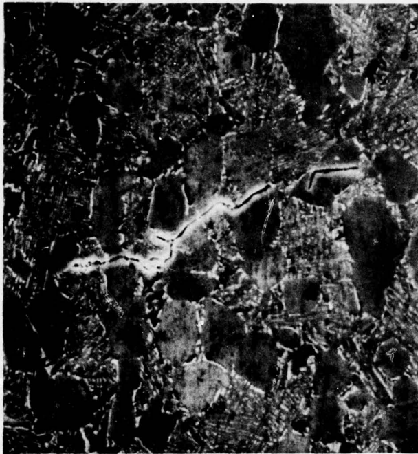
FIGURE 10. SEM MICROGRAPH OF 125 \mu\text{m} LONG SURFACE MICROCRACK USED IN SCOD MEASUREMENTS ON SAMPLE 7 (1000X)
