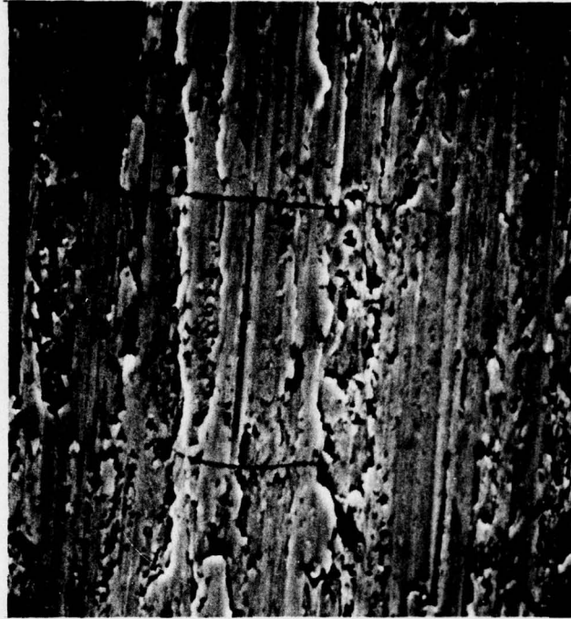
FIGURE 14. SEM MICROGRAPH OF SURFACE MICROCRACKS USED IN SCOD MEASUREMENTS ON SAMPLE 8. Labeled Crack 2 (1000X).
