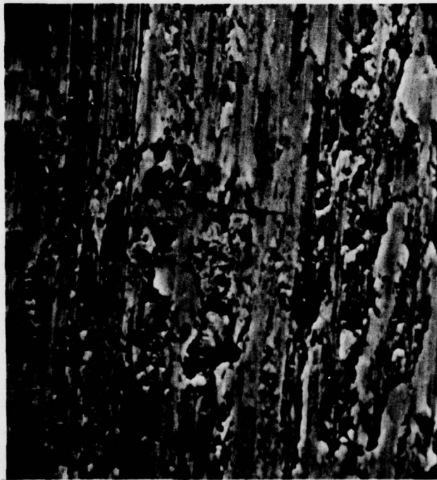
FIGURE 17. SEM MICROGRAPH OF SURFACE MICROCRACK USED IN SCOD MEASUREMENTS ON SAMPLE 8. Labeled Crack 6 (1000X).
