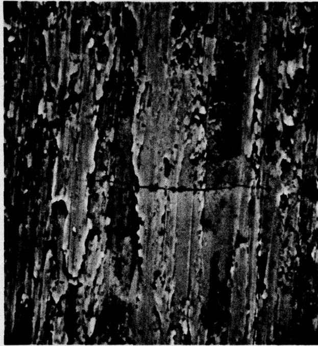
FIGURE 16. SEM MICROGRAPH OF SURFACE MICROCRACK USED IN SCOD MEASUREMENTS ON SAMPLE 8. Labeled Crack 5 (1000X).
