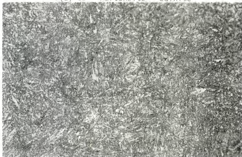
6(b) Mid-wall - Martensite - Bainite
