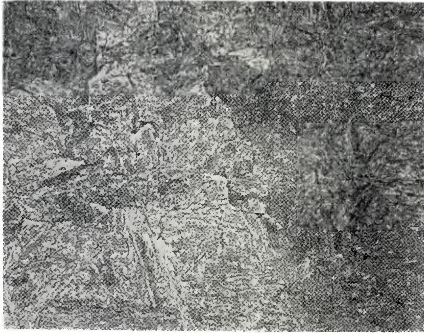
FIG. 4 - Microstructure at mid-wall of reheat treated rotary forged hollow ESR cylinder (Top) - 100CX (See Table 2)
