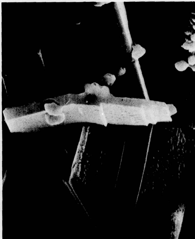
Enlargement of area indicated by arrow in previous photo, X2000. Illustrates complex crystal intergrowth and stair-stepped surfaces. Negative 06 09 76-11.
