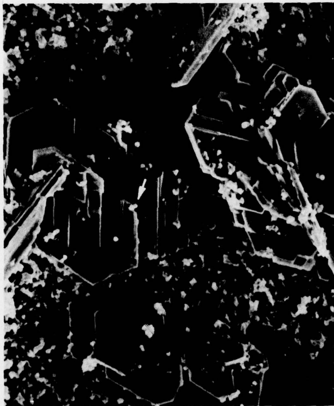
Typical crystal growth on formed surfaces of Panther Creek smectite-lime mixture, X330. Age of mixture is about 14 months. The arrow points to the area shown in the next picture. Negative 06 09 76-5.
