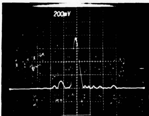
Fig. 2. The magnitude of the output signal for uniform illumination of the sensor.
