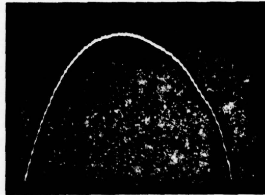
Fig. 4. Frequency response without CdS on LiNbO 3 . 2.5 dB/div. Frequency scanned 26–34 MHz.
