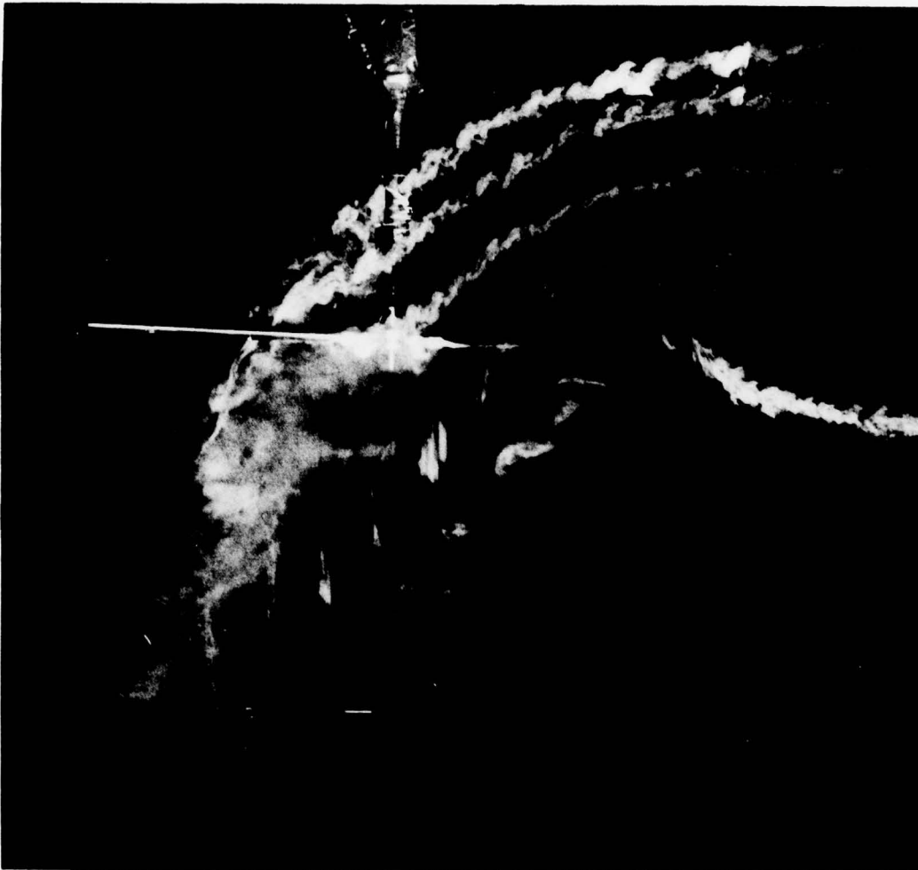
Figure 20. Smoke Flow Visualization Photograph of Wake Cross Section for Isolated Rotor in Low Speed Flight ( v = 15 kts).
