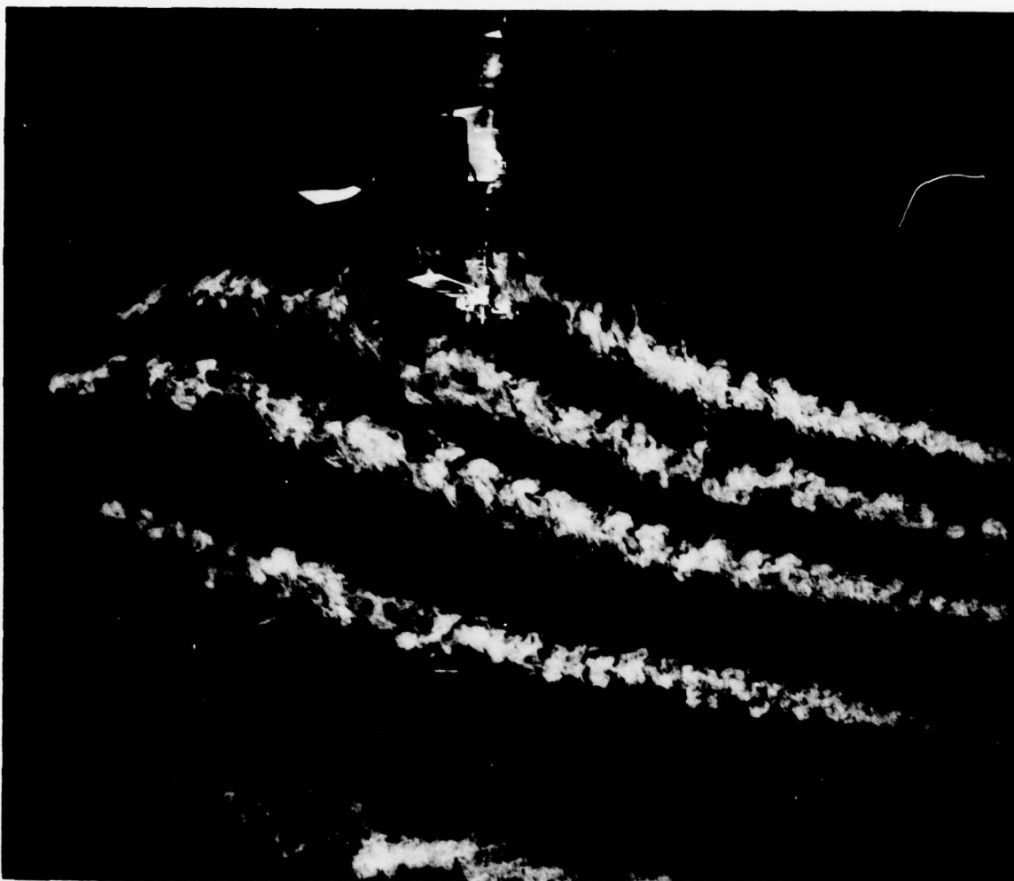
Figure 25. Smoke Flow Visualization Photograph of Roll-up of Lateral Wake in Low Speed Forward Flight.
