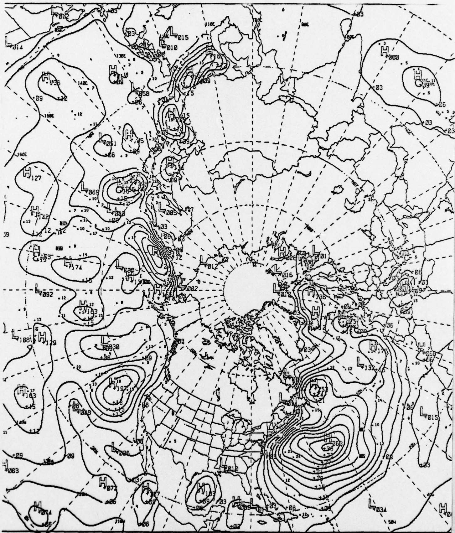
Figure 17 FIBWH analysis of significant wave height for 06Z 31 JAN 79 No. of reports: 297
