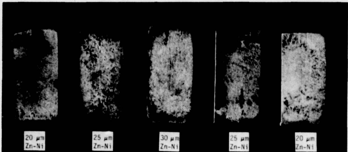
Figure 3. Specimens After 12 Days of Salt Fog (Specimen Size: 1.3 x 2.5 x 0.5 cm)
