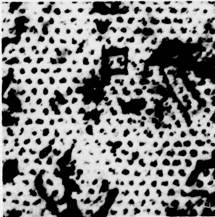
Fig. 7 Representative void structures in irradiated Mo and TZM: (a) Mo, imaged with a [111] beam direction showing void ordering; the voids appear dark due to a combination of overfocus and strain contrasts; (b) TZM, in which several coalesced voids can be seen.
