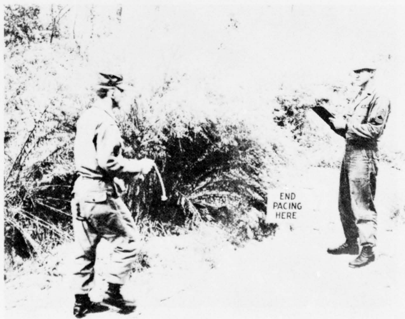
Figure 4. By Means of a Pace Course the Individual Soldier Determines His Standard
