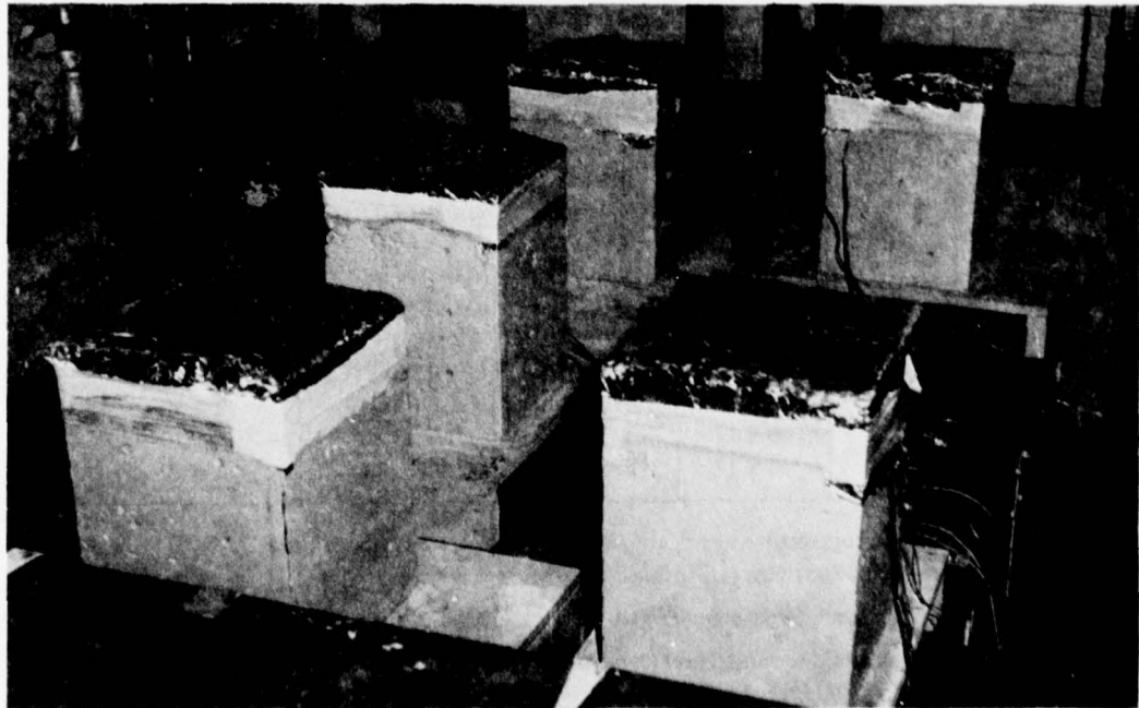
Figure 4. Prismatic slab-type specimens being cured.
