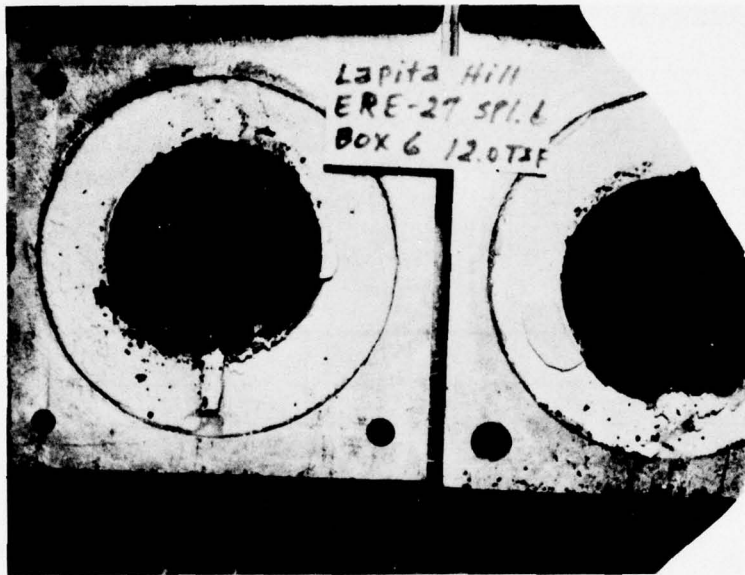
c. Single-plane direct shear test after failure at 12- tsf normal load
