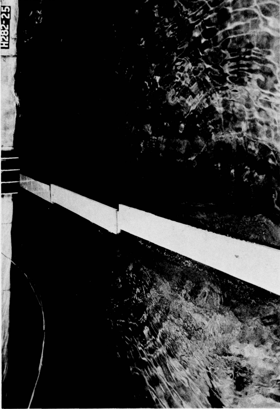
Photo 27. Overhead view of Plan 1 in the 75^\circ linear configuration under attack of 3.0-sec, 2.0-ft waves in a water depth of 25 ft
