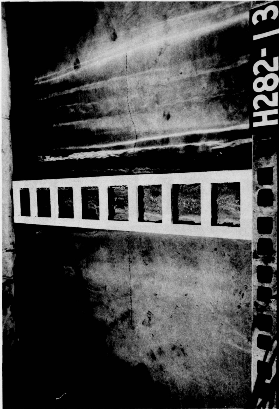
Photo 20. Overhead view of Plan 3 under attack of 2.5-sec, 2.0-ft waves with anchor chains uncrossed
